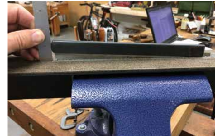
Remove the handle and clamp the plate/back assembly in the jaw extenders, leaving ½in clearance at the toe with the heel making positive contact on the surface of the jaw extenders
