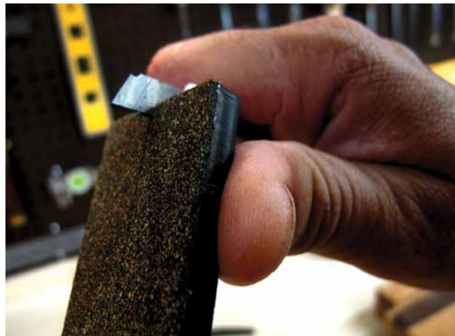
Use a craft knife to open up a slot in the prybar
