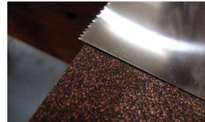
Once you've peeled off your sawback, remove the plate from the jaw extenders and lay it (teeth up) on one of the saw vice pieces with ½in to ¾in of the toothline exposed...
