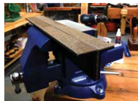
Angle iron jaw extenders for your mechanic's vice
