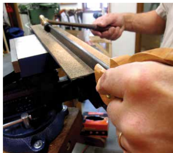
Gently tap the folded back towards the handle to close up any gaps
