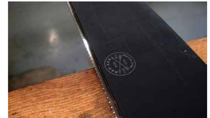
...then sandwich the plate with the other half of the vice; secure both ends and inch-down with c-clamps
