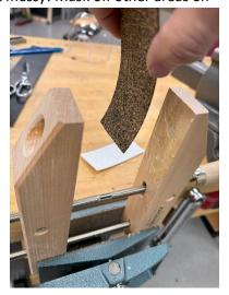
**Step 4:** Close the jaws of your clamp with plastic tape or a plastic bag in between to prevent the strips from gluing onto one another—the cork rubber is a bit porous and you don't want the spray adhesive to
