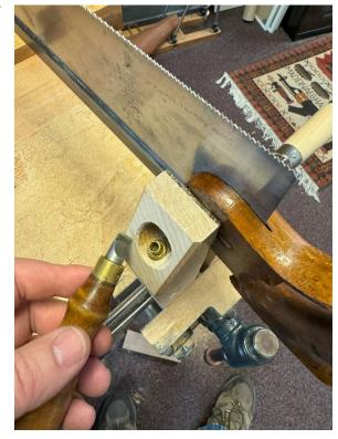
store, bore a 7/8" diameter hole, line inside of the jaws with cork rubber you can purchase from <a href="McMaster-Carr">McMaster-Carr</a>, clamp your saw handle inside the jaws, then unscrew the frozen nut through the access hole you've bored. You see—the hole allows you access to the slotted head of the nut (or bolt,
