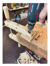
**Step 6:** Now remove the cork rubber covering the bore hole without damaging the cork rubber on the opposing jaw. This is where your 7/8" router bit comes into play. Widen the jaws enough to clamp onto your bench over a sacrificial piece of wood. Chuck your router bit into a drill and drill through the hole you bored earlier with the spade bit
