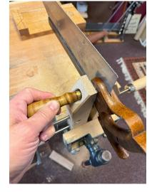
**Step 8:** Mount your saw into the clamp, such that the frozen slotted nut/bolt is exposed in the hole you'll access with your screwdriver. Ensure the jaws remain parallel to one another as you tighten the clamp; this will maximize clamping pressure right where you want
