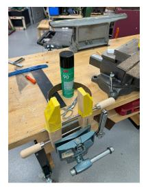
**Step 3:** Now you're going to line the inside jaws of the clamp with cork rubber. Even though adhesive cork rubber is available, the adhesive will wear out and the cork rubber will begin peeling off. To prevent this, I like spray 3M adhesive spray onto the area inside the jaws where the cork rubber strips will do. Mask off the exterior part of the clamp with painters or masking tape to avoid spraying where you don't want the adhesive—it can get messy! Mask off other areas on
