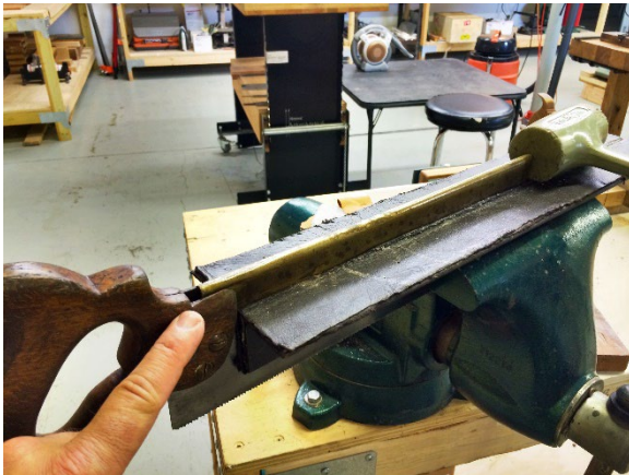
Figure 2: Cut some 1.5" or 2" angle iron to 18" sections, smooth the metal, and line it with leather or cork-rubber-- and now you have a superb vise accessory with which to grip your plate when adjusting or removing a sawback.
