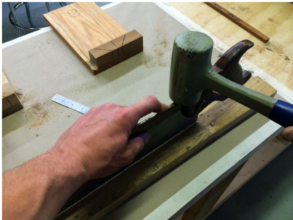
Figure 3: Lightly tap the heel end of the sawback while clasp the underside of the sawback with thumb and forefinger. You'll know when the back shifts upon tapping it.
