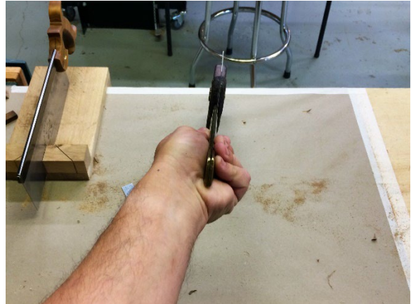
Figure 6: Always, always, always assess what you've done with each step and don't rush it. You know you've created an S-roll--so take the time to see it. Then retension it away.
