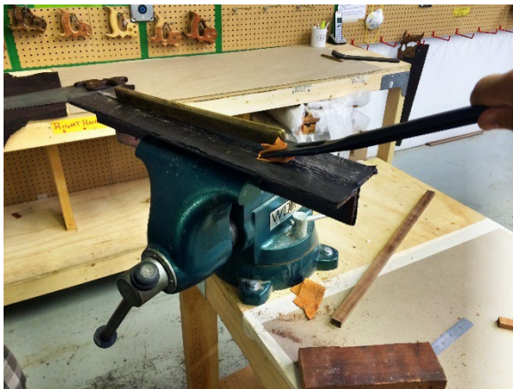
Figure 5: lift your sawback with a simple 14" x 1.5" x 1/4" flat iron bar with a kerf sawn 2.5" down on-center at one end of the bar. Line about six inches of it with cork-rubber, and now you've made yourself a sawback lifter.
