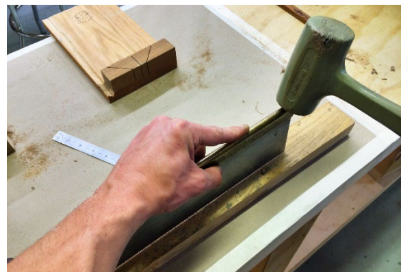
Figure 4: Repeat the process at the toe end, again, while using your thumb and forefinger to ascertain whether your back shifts.
