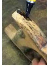
Using a stain marking pen to blend in the grafted wood with the original wood
