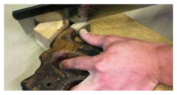
Secure your handle onto a bench hook or clamp and literally saw off the big chunks to rough form
