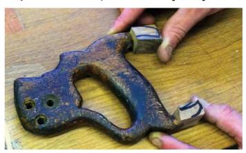
Trace out the horn outline on your graft wood and cut the squares proud of the trace for length, thickness and width
