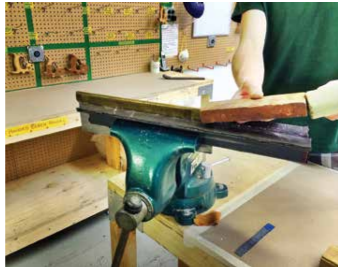
Shoving the sawback forward of the toe end of the plate to create an air gap
