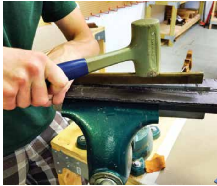
Tapping the sawback onto the toe end of the spine and tapping it on with a light dead-blow mallet
