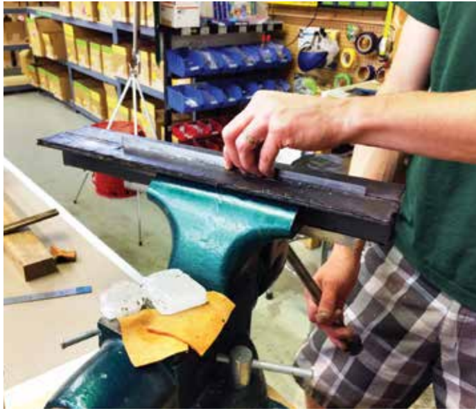
Mount the sawplate tightly into the pair of leather-lined angle iron pieces and clamp in your vice
